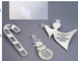
Mirrored acrylic is also a good substrate for laser cutting and can create some unique results. The plastic reflective coating on the mirrored acrylic will be vaporised during the cutting process, so it
