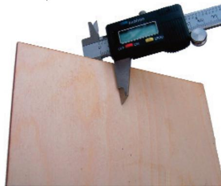
The original design was made to fit .124" thickness materials. If we select everything in the design and proportionally change the size it will go together perfectly. Let me show you what I mean. The new plywood I just bought measures out at .133" thick, so I
