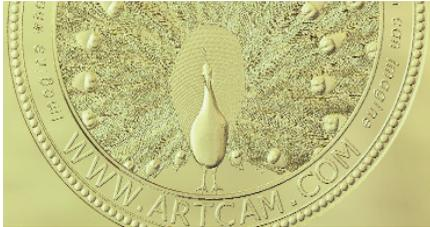
The peacock was then brought in from the 'Clipart Library', scaled to size and pasted down onto the model. To stop it from overlapping the circular edge, the nearest vector was selected and using the 'Shape Editor', all of the peacock design that passed beyond the selected vector was levelled.
