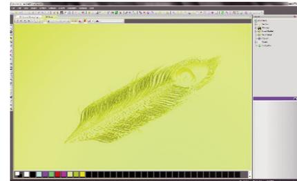
Using the image as a guide, the drawing tools were used to create the spine of the feather and the shape of a feather strand. Using the 'Shape Editor' a domed shape was added to the vectors. To make this a more fluid shape, 'Node Editing' was used. This allows designers to add or alter points in the vector to alter its shape. The base of the feather was then smoothed out, so that it would not stand proud of the feather spine when added to it.
