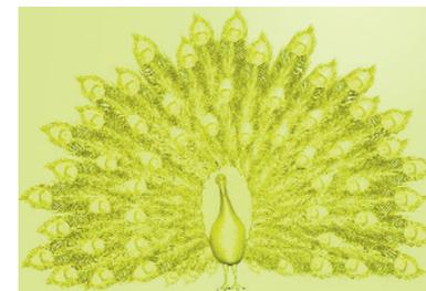
This only left ArtCAM designers to assemble the final peacock design. All the previously created 'Clipart' was dragged in from the 'Clipart Library' into one ArtCAM model. With ArtCAM's 'Free Relief Modelling' process they could all be kept open at the same time to ensure that all the pieces were the correct size and fitted together properly before they were pasted down onto the relief. As with all other models, this was then saved into the 'Clipart Library' for future use.
